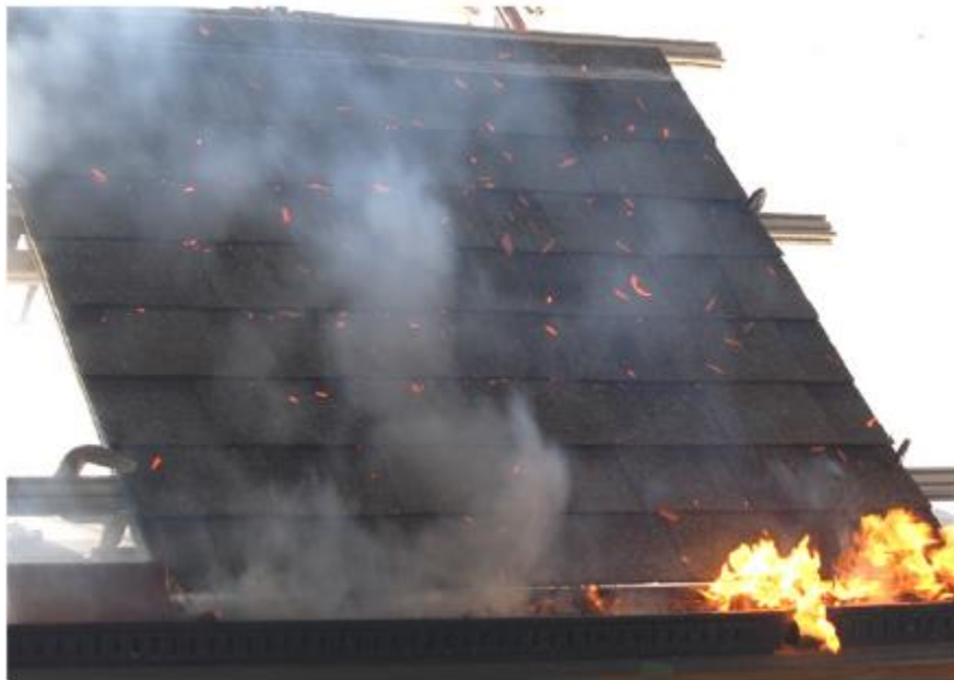
Figure 18: Ignition of pine needles in a gutter after transitioning to flame spread from (Manzello et al., 2008). This fire did not actually ignite the roof assembly, but there is potential for ignition of the roof assembly depending on the gutter, roof and flammable material inside the gutter.
