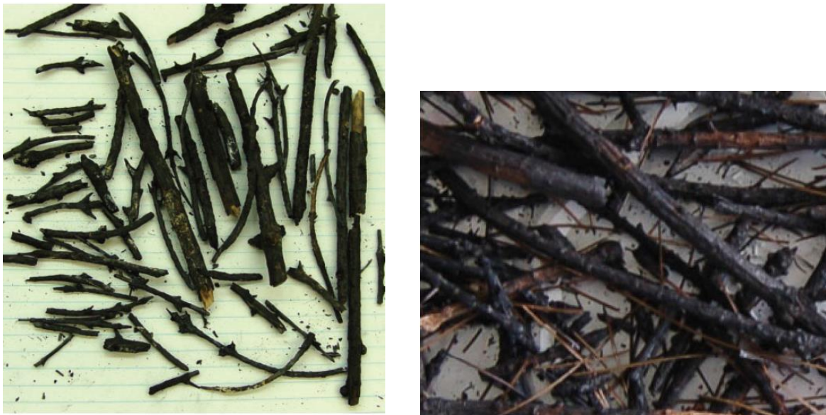
Figure 8: Digital photographs showing samples of the firebrands collected as a function of tree size and moisture content. (left) Douglas-fir with tree height 5.2 m, moisture content 20%. From (Manzello et al., 2007). (right) 4 m Korean Pine with moisture content 13% (Manzello et al., 2009).
