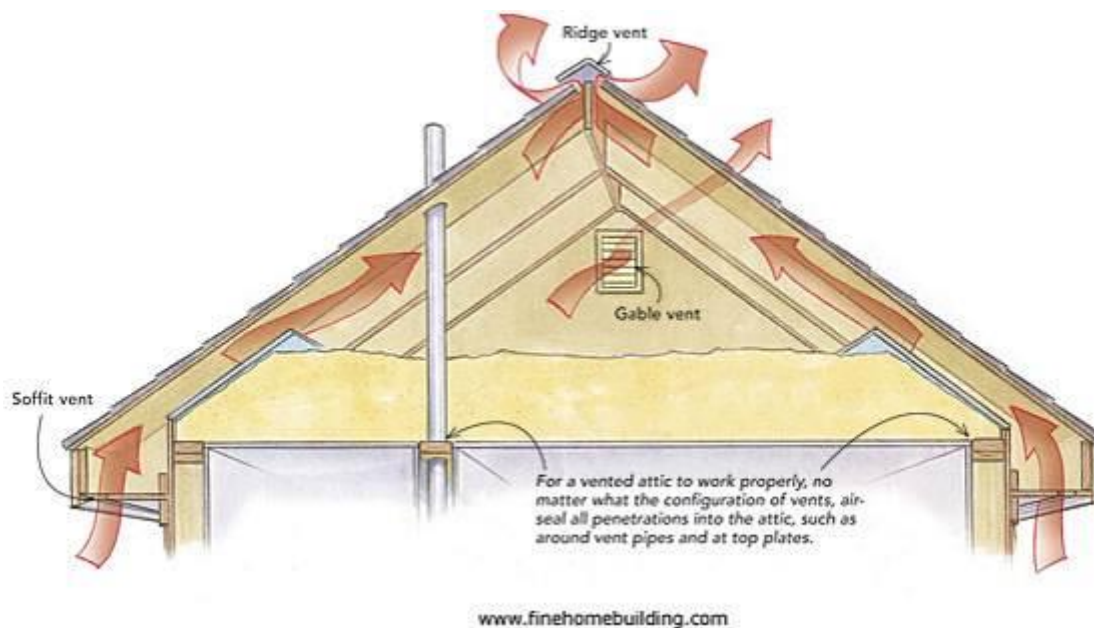
Figure 21: A schematic of vents used to ventilate an attic space from www.finehomebuilding.com . It is common to have at least one outlet vent type, for example gable, ridge or soffit.
