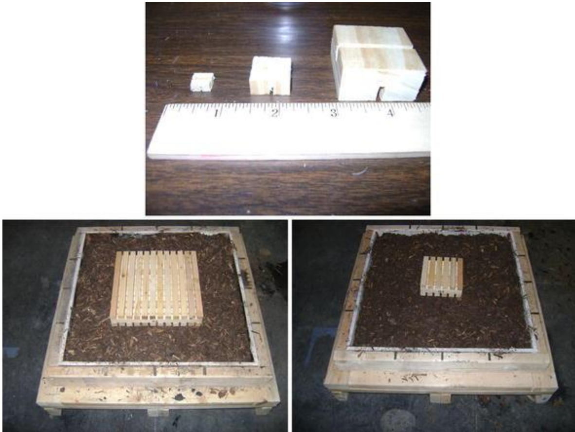
Figure 20: Mulch bed tests from Beyler et al. (2012) showing 1/4, 1/2 and full-size Class C brand ignition sources from the ASTM E-108 test.
