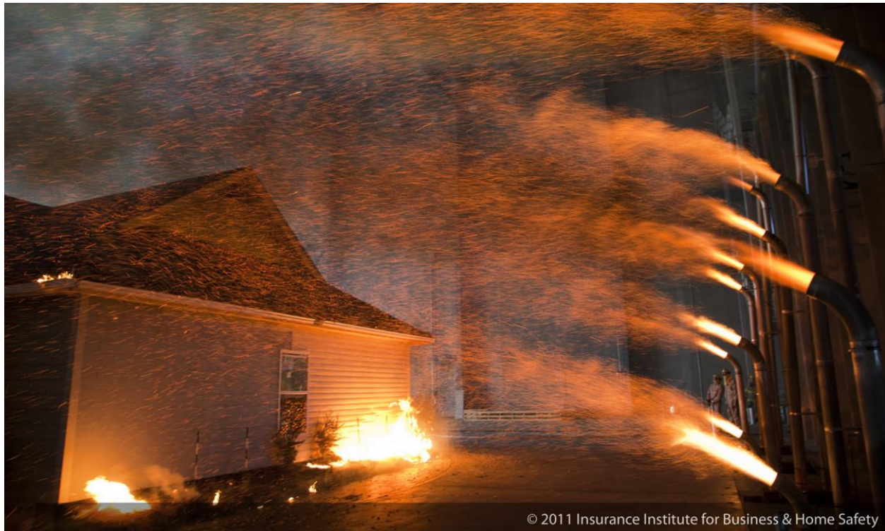
Figure 15: Ember storm produced in the IBHS research facility (IBHS, 2014).
