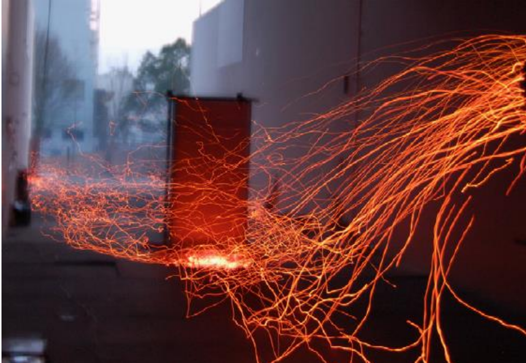
Figure 24: High-exposure time photograph showing firebrand accumulation in front of an obstacle from (Manzello et al., 2012a).
