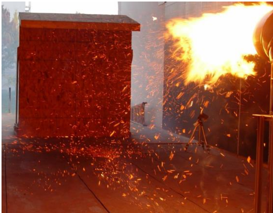
Figure 14: A typical experiment with the NIST Dragon in BRI's FRWTF (Manzello, 2014).
