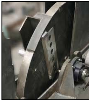
Top: A drum style Chipper. Bottom: Disc chipper wheel
